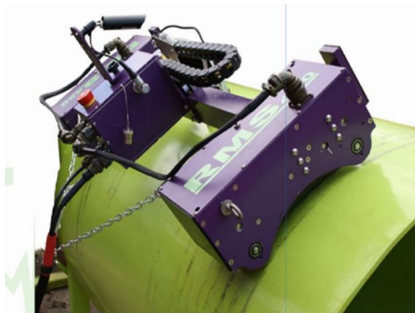
Fig. 2. Ultrasonic equipment fixed to the external wall of the pipe
